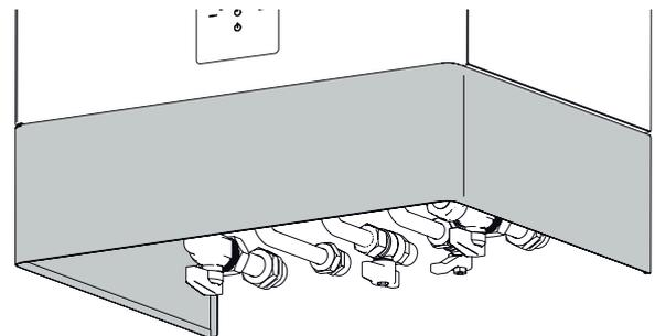
fig. 6 - Fittings cover kit assembled
