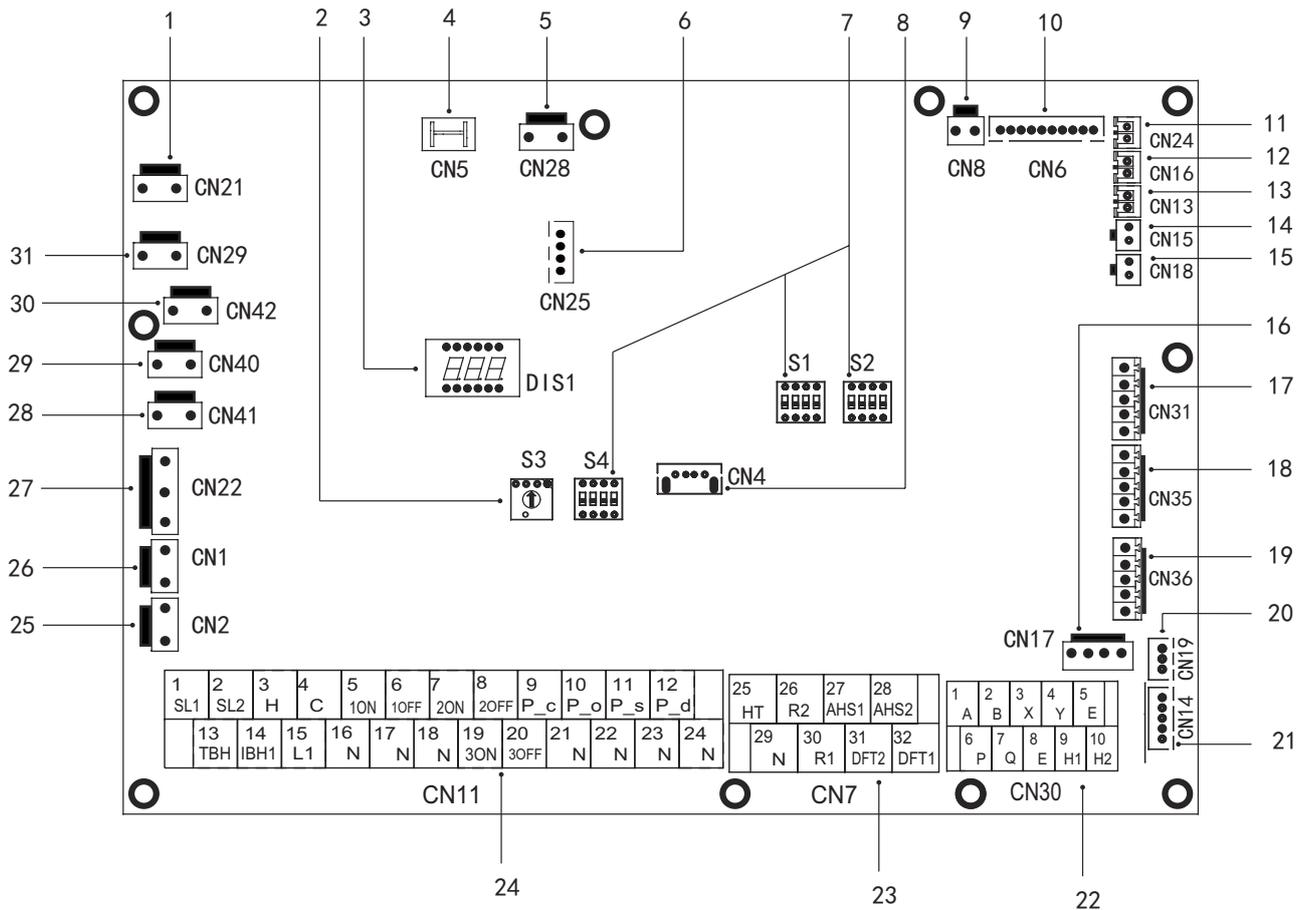
fig. 34 - Detail of heat pump hydronic board
