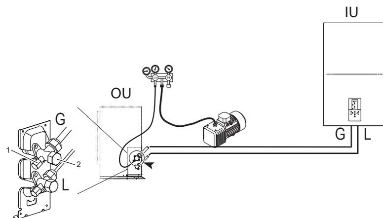
fig. 18 - Air purge with vacuum pump
