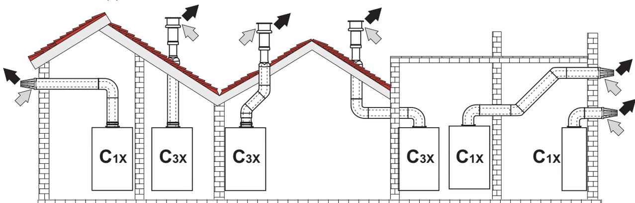
fig. 19 - Example of connection with coaxial pipes (
