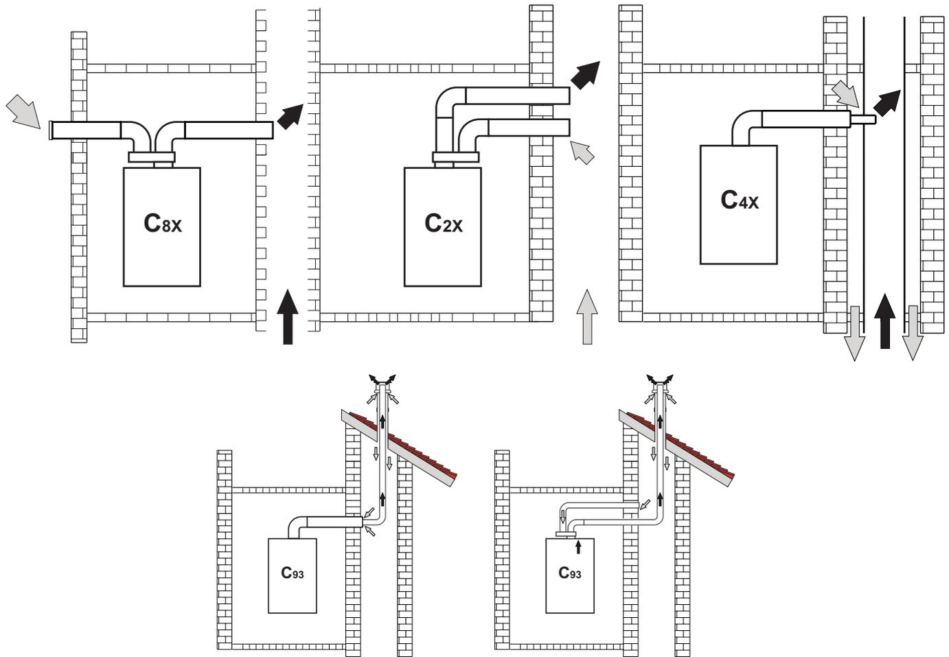
fig. 25 - Example of connection to chimneys (☞ = Air / ☛ = Fumes)
