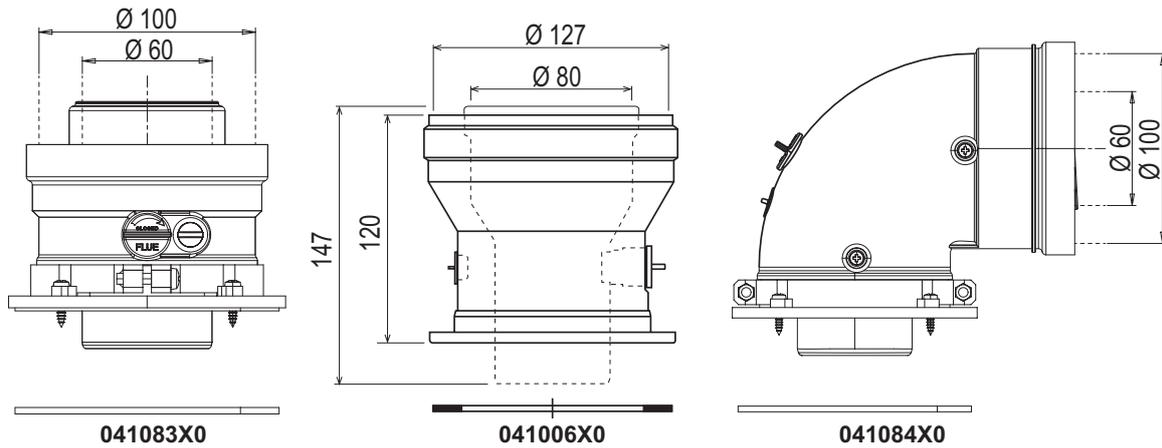
fig. 20 - Starter accessories for coaxial pipes
