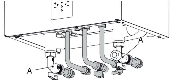
fig. 4 - Assembled hydraulic kit
