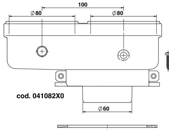
fig. 22 - Starter accessories for separate pipes
